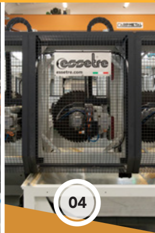
04 PERIMETER FENCE FOR EACH SAW BLADE UNIT
