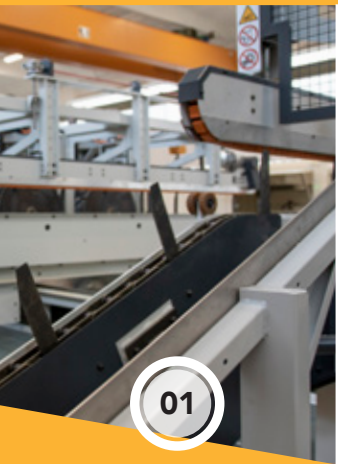
01 THRU-FEED CHAINS FOR 2X WITH "DOGS"
